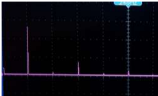
Fig. 8. Spectrum of Sinewave
