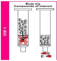
Rinse the packing with a small volume (typically 200µL to 2mLdepending on the tube size, or 5-10mL depending on the disk size) of a solution that removes compounds of interest.
