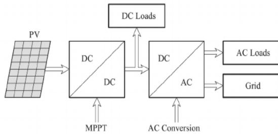
Fig. 4. Block Diagram Representation of Photovoltaic System
