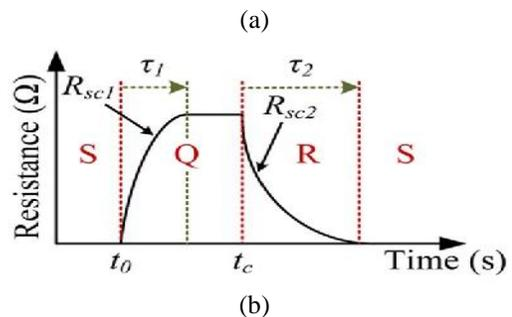
Fig. 3. SFCL Performance Evaluation Graph Indicating the Relationship between SFCL Impedance and Reduction in Fault Current
