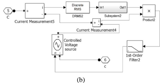
Fig. 2. Single phase SFCL model developed in Simulink/Sim-PowerSystem
