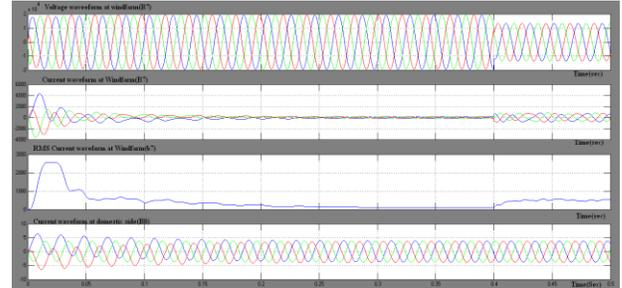
Fig. 13. Fault2 with SFCL at Location1 & 4
