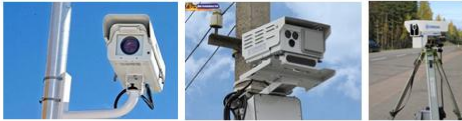
Figure 1; CCTV cameras and photoradar vehicle detector complexes
