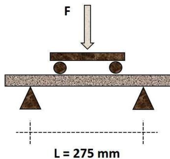
**Figure 2.** Schematic diagram of three-point flexural test<sup>[2]</sup>
