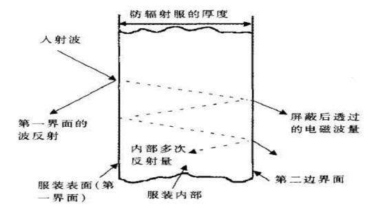
In the refraction and reflection theory of electromagnetic waves, we have the simplest vertical incidence as an example. According to the Fresnel principle, both the vertical polarized wave and the parallel polarized wave transmission coefficient are
