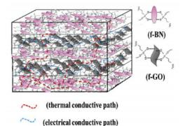
Figure 3. Thermal and electrical conductive schematic of the ordered multilayer film[27].
