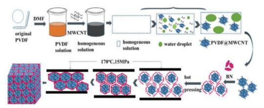
Figure 2. Preparation process of PVDF @MWCNT composites<sup>[26]</sup>.
