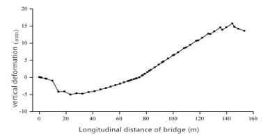
Figure 3. Influence of unbalanced weight of boom beam on linear shape of main beam.
