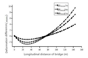
Figure 4. Influence of the distribution length of the weight on the linear shape of the main beam.
