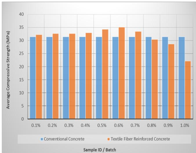
Fig. 7: Compressive strength of concrete at 28 days with various percentage of textile waste compared to normal concrete
