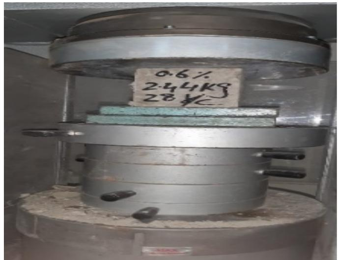
Fig. 5: Compressive strength test
