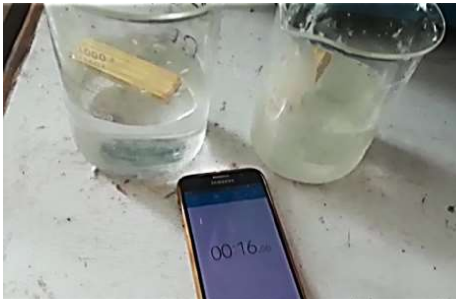
Figure 6. Initial image of water absorption.
