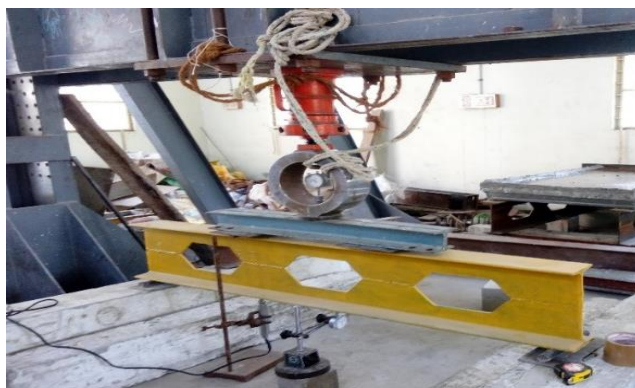
Figure 4.1 Test setup for castellated beam
