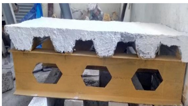
Figure 3.6 Deck system after concreting
