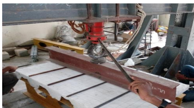
Figure 4.3 Test arrangement for composite slab
