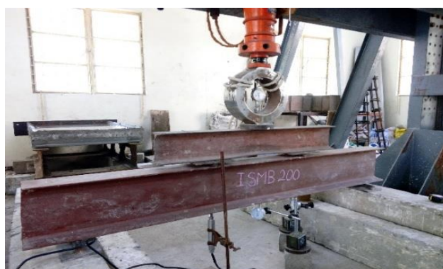
Figure 4.1 Test setup for castellated beam
