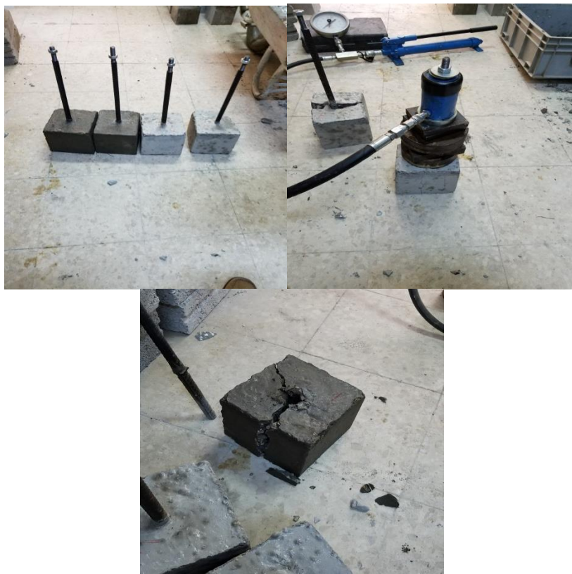
Figure 3-a Bond Stress Test for Specimens in Fresh Water and Dead Sea Water.
