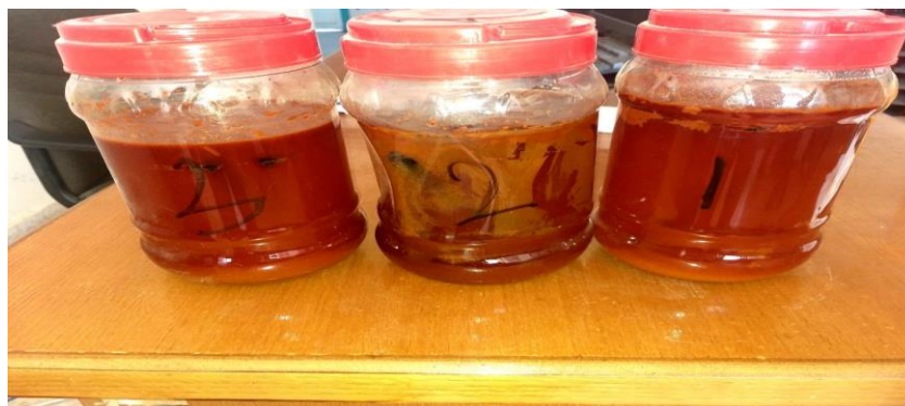
Figure 4: Corrosion of Steel Bars under immersion in Dead Sea water jar.
