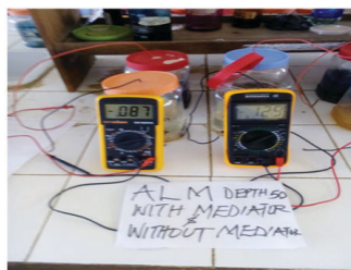
Plate 1: MFC Chamber showing River Ala mud surface and depth 50 cm with mediator and without mediator
