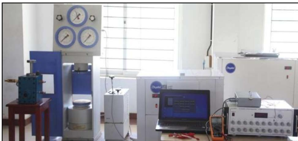
**Figure 2** Laboratory triaxial test setup for frozen soil
