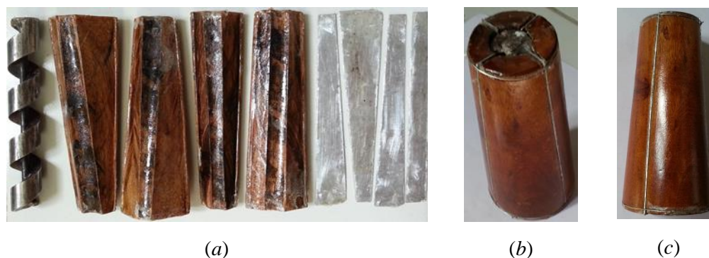
Figure 2 Mandrel of \alpha = 5^\circ configuration: (a) parts, (b) assembled mandrel isometric view, (c) assembled mandrel front view.
