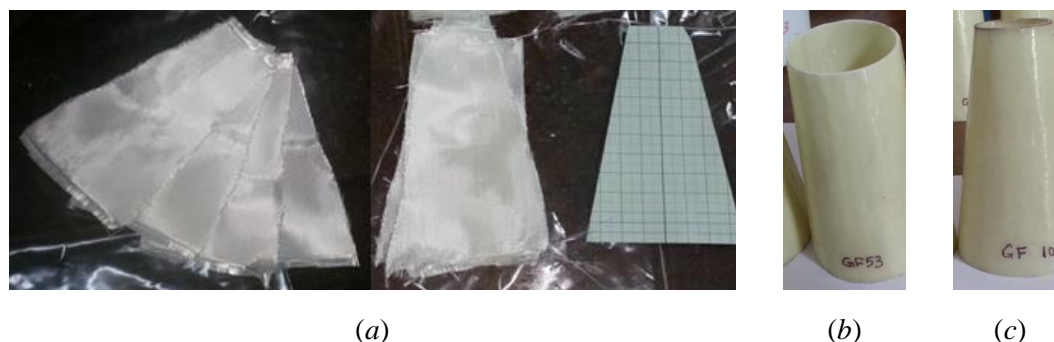
Figure 1 GFRP frusta: (a) woven glass fibre cuts, (b) specimen with \alpha = 5^\circ , (c) specimen with \alpha = 10^\circ .
