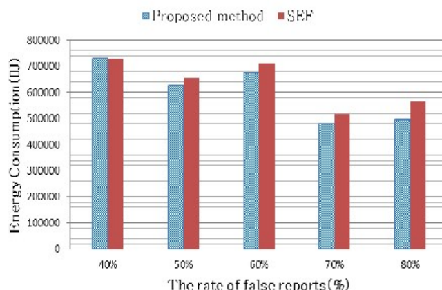
Figure 15 Energy consumption versus the rate of false reports (Fraction of compromised nodes =4)
