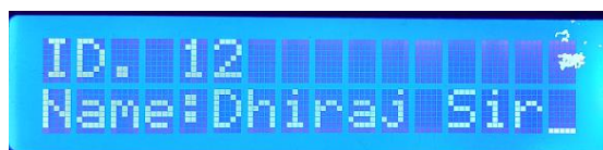
Figure 13 Faculty ID and Name are displayed on LCD when Faculty fingerprint matches at the start of the session
