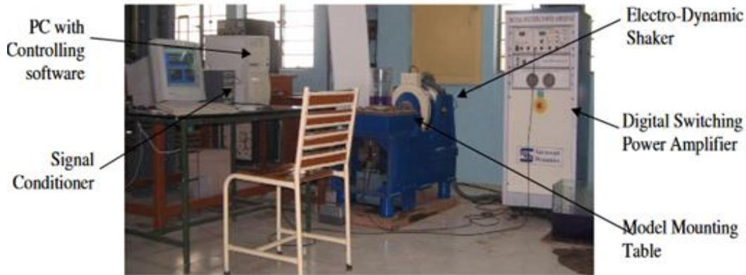
**Figure 3.**Experimental set-up-shake table test
