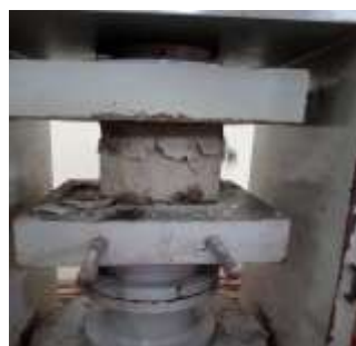
Figure 3 Compressive testing in CTM
