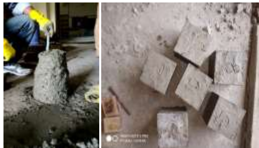
Figure 2 Fresh concrete slump and cubical specimens after 28day curing
