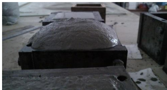
Figure 1 Final stage after hydration of aerated concrete occurred
