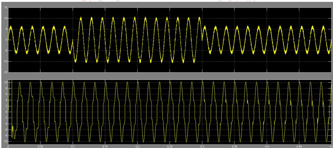
**Fig.2 IS/IL Load during SAG**
