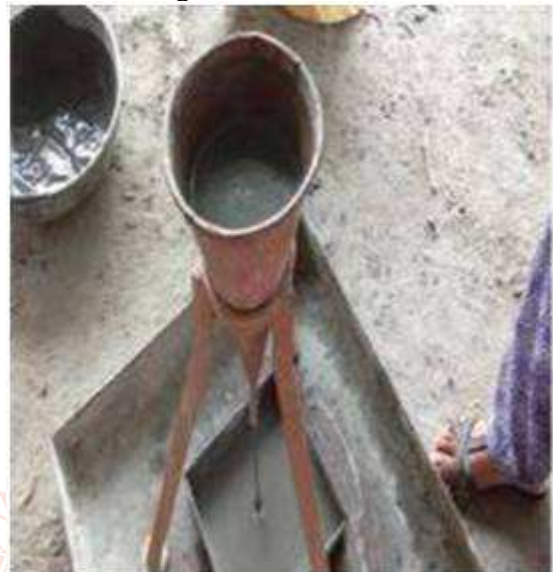
Fig1. Marsh cone test
