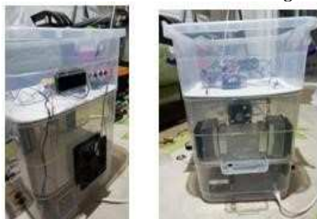
Figure 7. The Ambient Humidity Stabilizer with Nebulizer and Dehumidifier
