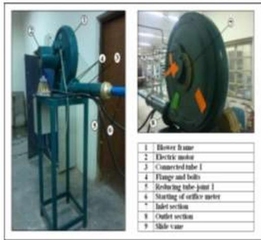
Fig.8, the photo of air blower system
