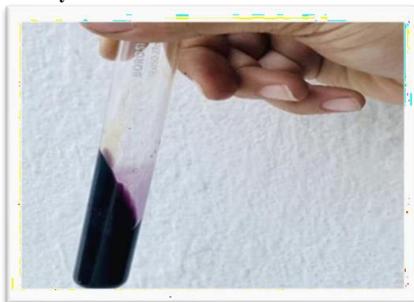
Fig. 5: Qualitative chemical test for extracted salicylic acid occurs purple color indicates the presence of salicylic acid.
