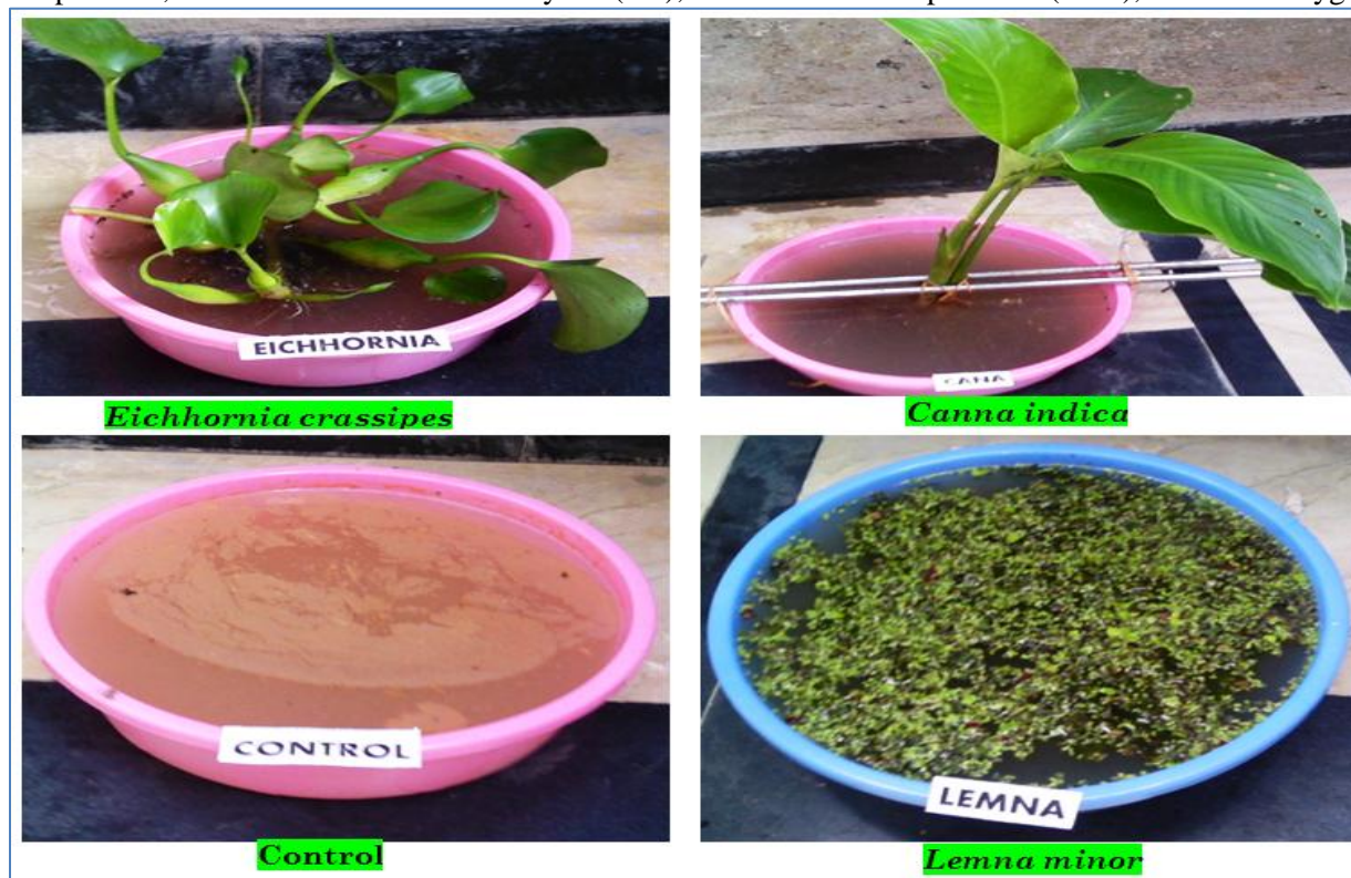
Fig 2. Experimental set up for treatment of sewage waste water by E. crassipes , C. indica , L. minor along with control.
