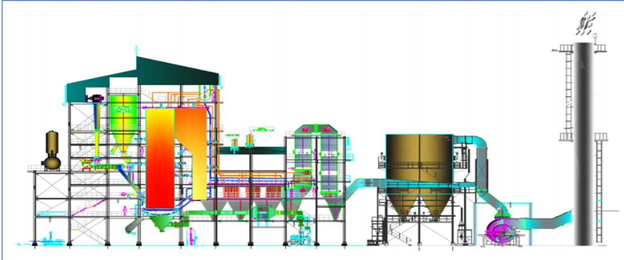
Fig 2. Diagrammatic representation of Spent wash/Vinasse Incinerator (Source: Balasubramanian and Kannan, 2016)
