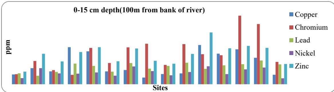
Fig 4. Metal concentration in soil 0-15cm depth (100m from bank of river).
