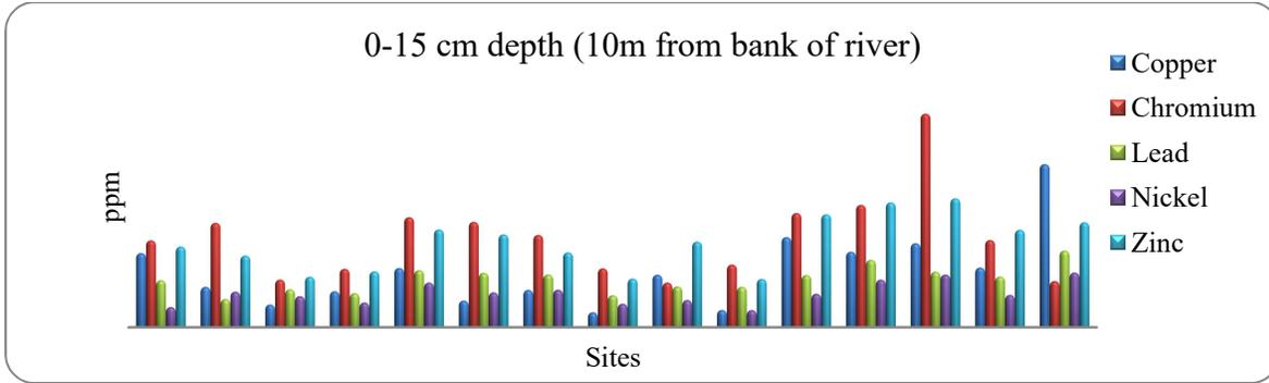
Fig 2. Metal concentration in soil 0-15cm depth (10m from bank of river).
