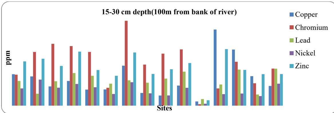
Fig 5. Metal concentration in soil 15-30cm depth (100m from bank of river).
