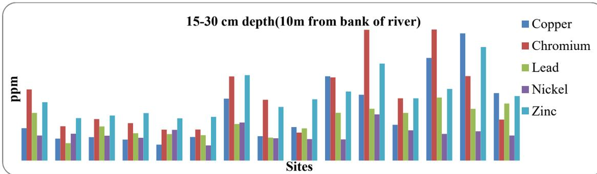
Fig 3. Metal concentration in soil 15-30cm depth (10m from bank of river).
