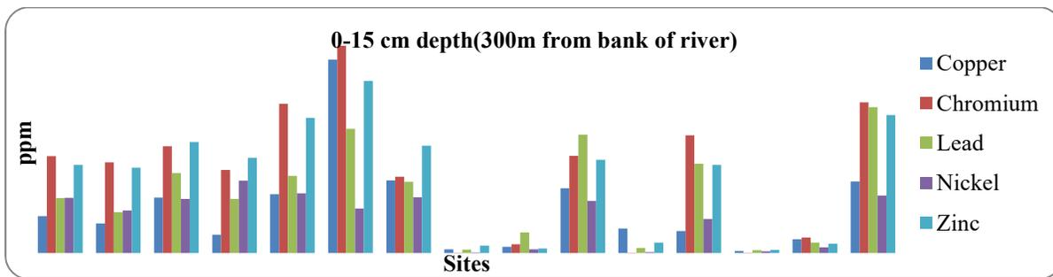
Fig 7. Metal concentration in soil 0-15 cm depth (300m from bank of river).
