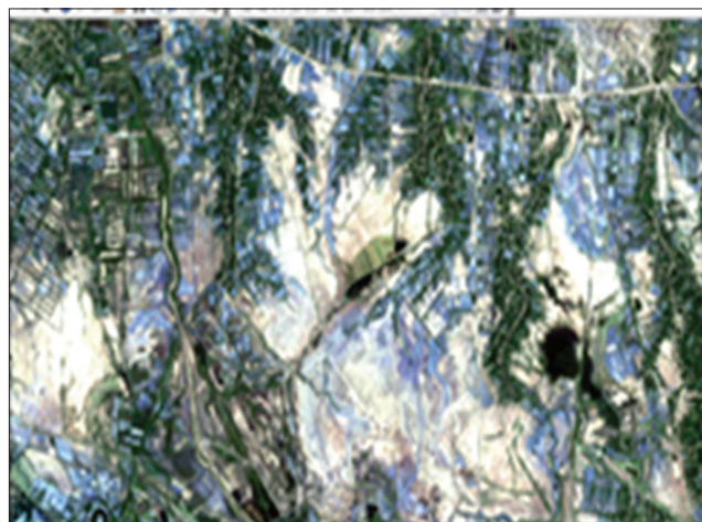
Figure 3: The combination of channels 3, 2, and 1 of the pilot plot in natural colors, areas of bright white and gray colors are very strongly and strongly saline soils
