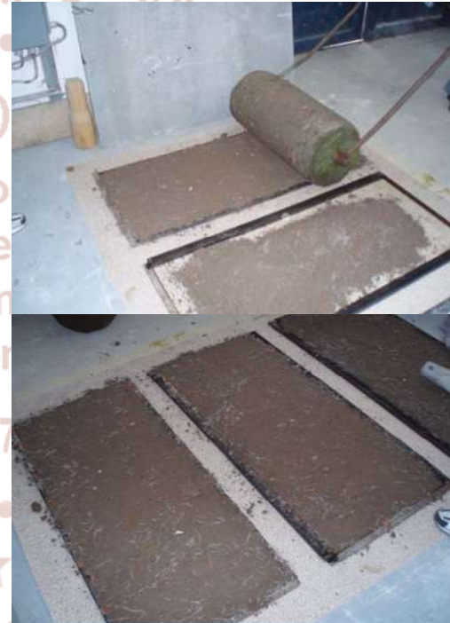
Fig. 3.2 - The Preparation of Slabs from Fibre Concrete
