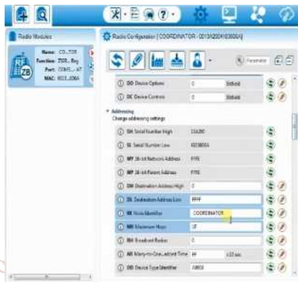
Figure3. XBee S2C Configuration as Coordinator
