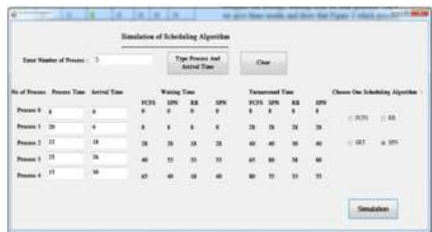
Figure 6: Comparison Waiting Time and Turnaroud Time for Four scheduling policies in Simulation 5.
