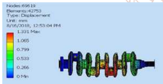
Figure 8: Displacement of Cast Iron
