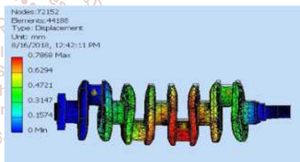
Figure 12: Displacement of Alloy Steel
