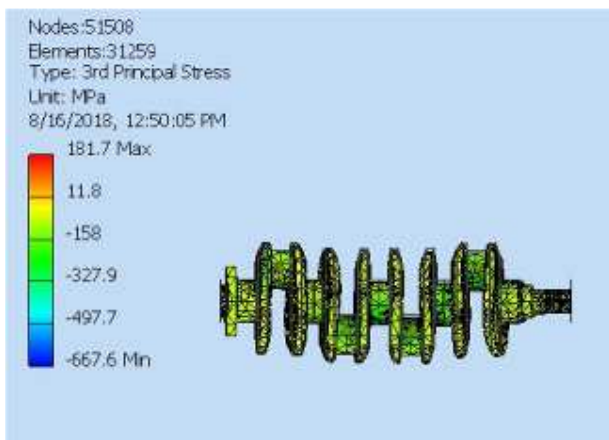
Figure 15: 3 rd Principal Stress of Carbon Steel
