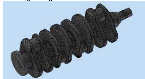
Figure 3: Meshed Modeled of Crankshaft
