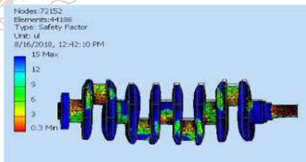
Figure 13: Safety Factor of Alloy Steel
