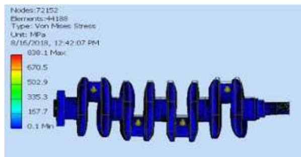
Figure 10: Von-misses Stress of Alloy Steel
