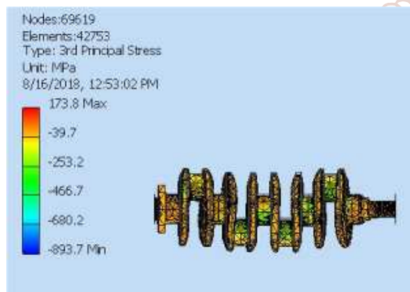
Figure 7: 3rd Principal stress of Cast Iron
