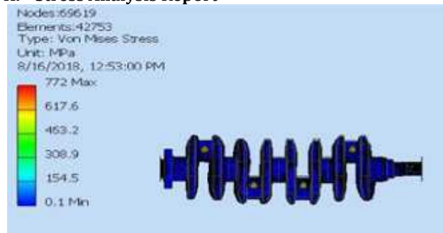
Figure 6: Von-misses Stress of Cast Iron
