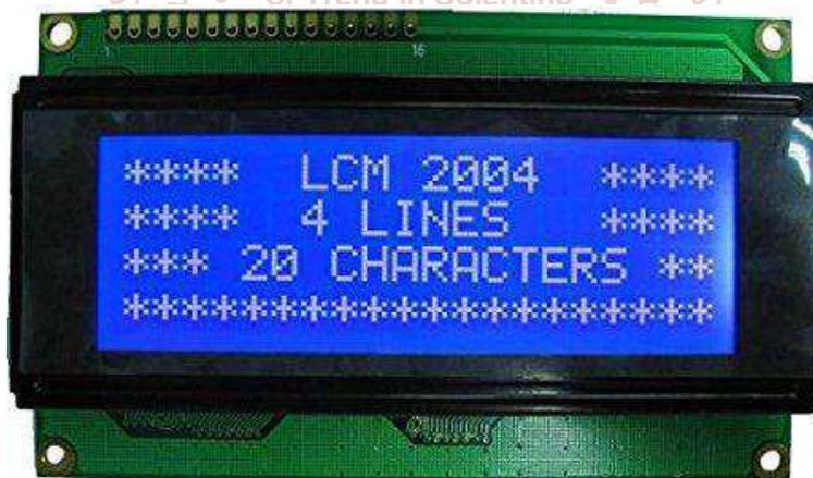
**Fig - 22 20X4 LCD Display with blue back light**
