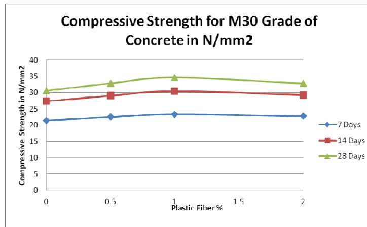
**Figure 1.2 – Compressive Strength of M30 Grade concrete**
