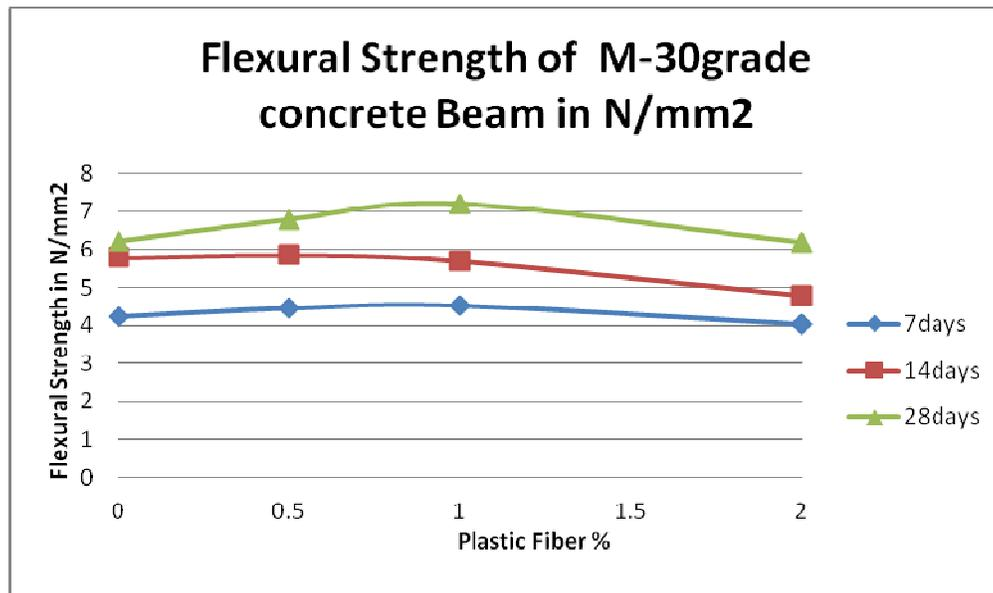
Figure 1.4 - Flexural Strength of concrete Beam
