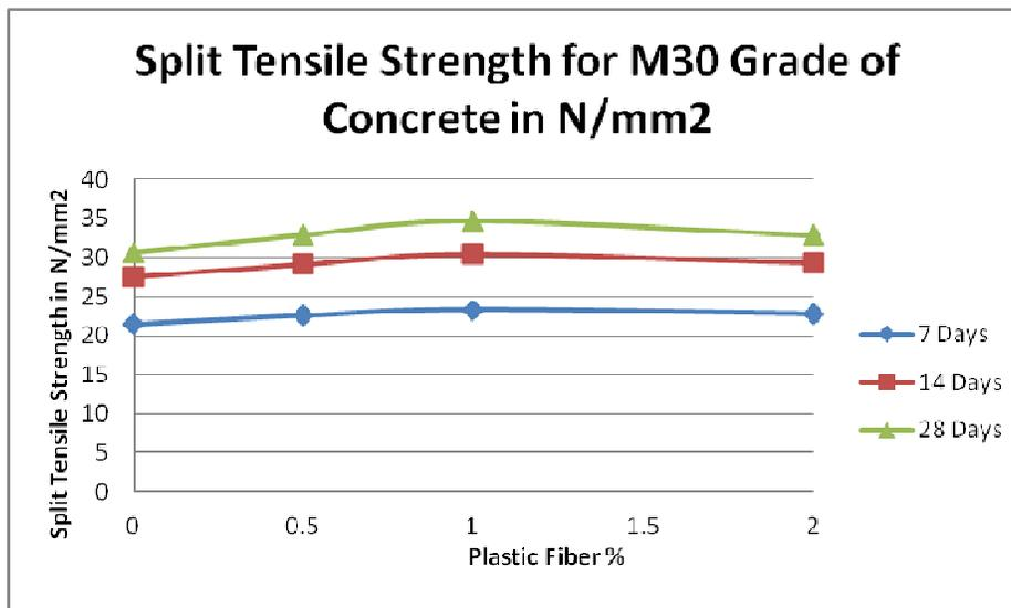
**Figure 1.3 Split tensile strength of Cylinder**
