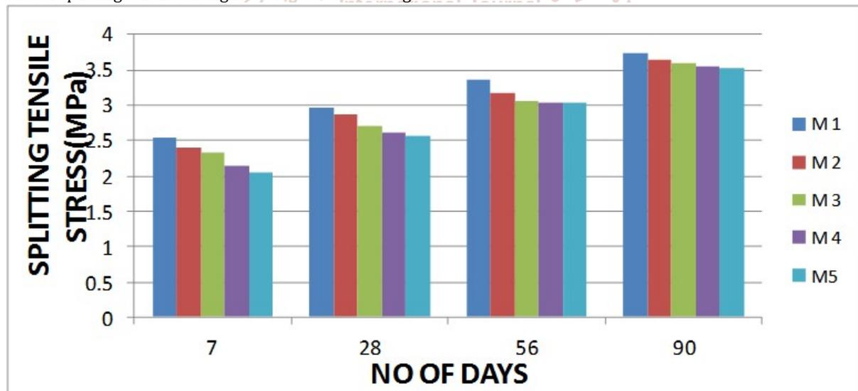
**Fig.: Splitting Tensile Strength of Concrete**
