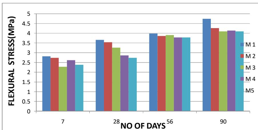
Fig.: Flexural Strength of Concrete
