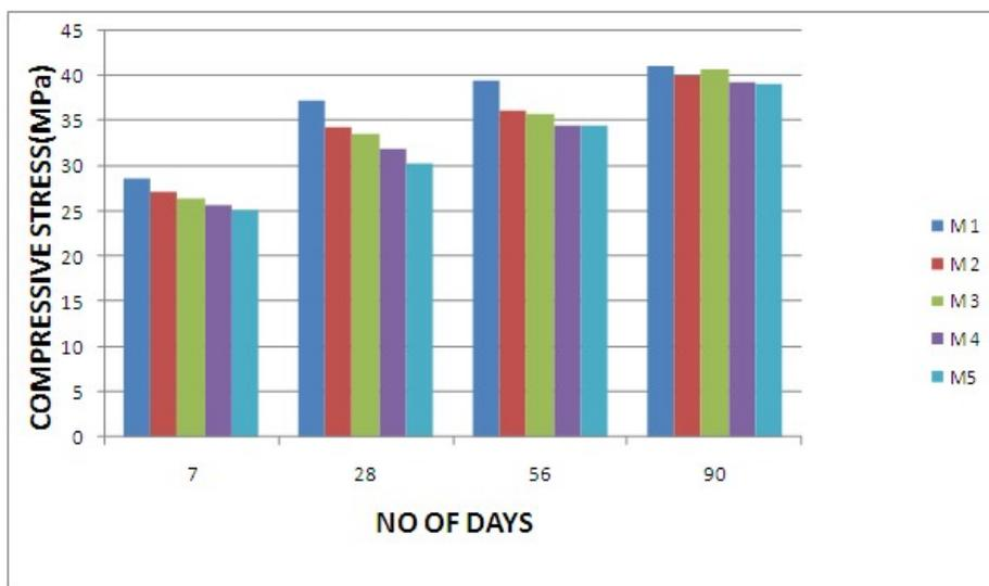
Fig.4.2: Compressive Strength of Concrete
