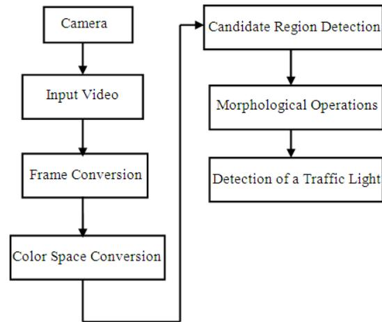
Figure2. Block Diagram of Traffic Light Detection
