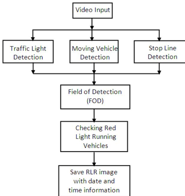
Figure1. Block Diagram of the automated red light violation detection system
