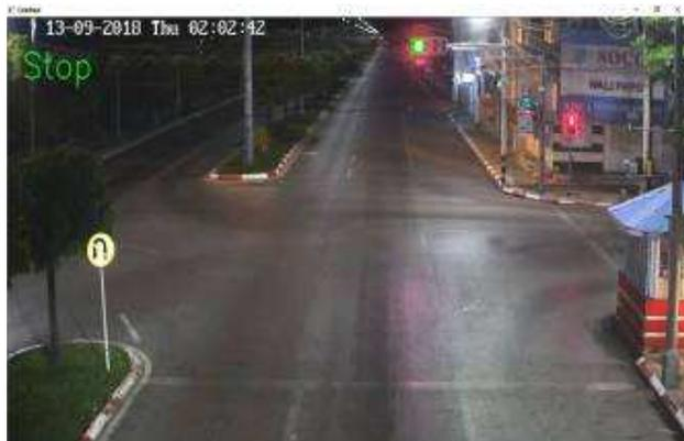
Figure8. Traffic light detection for red color
