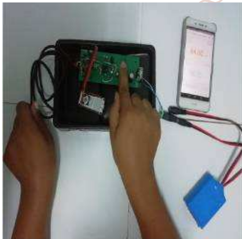
Fig. 7 Testing IoT Based Healthcare Monitoring System with Thingier.io Cloud
