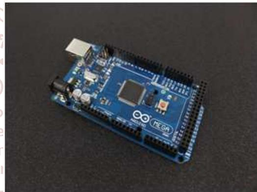
Fig.3. Arduino Mega
