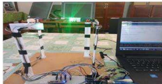
Fig.7. Traffic light with regular timing sequence
