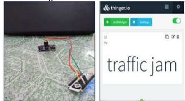
Fig.5. Testing ultrasonic sensor and sending to the thinger.io
