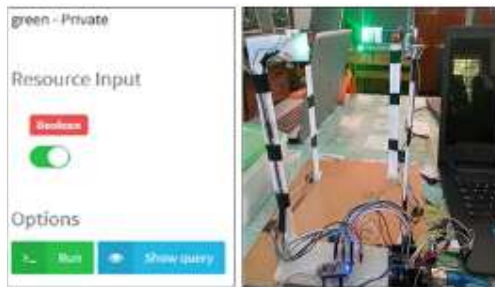
Fig.8. Controlling timing sequence of traffic light from thinger.io
