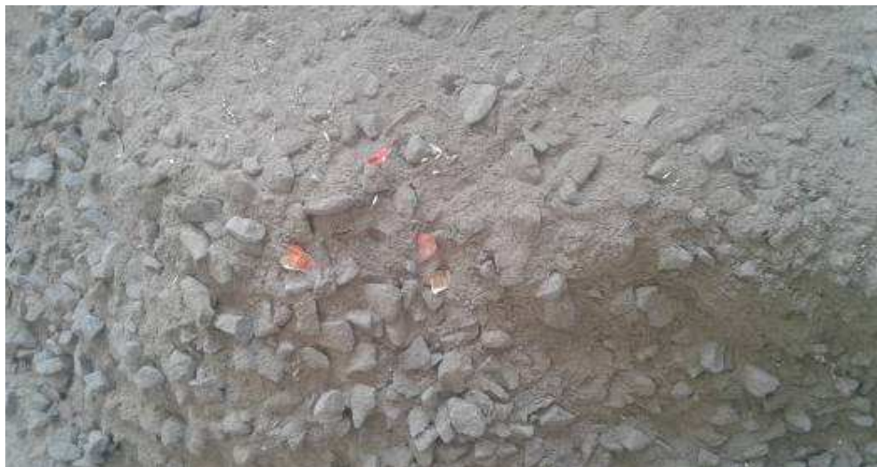
Fig. No. 3.1: Fibres added concrete mix before adding water
