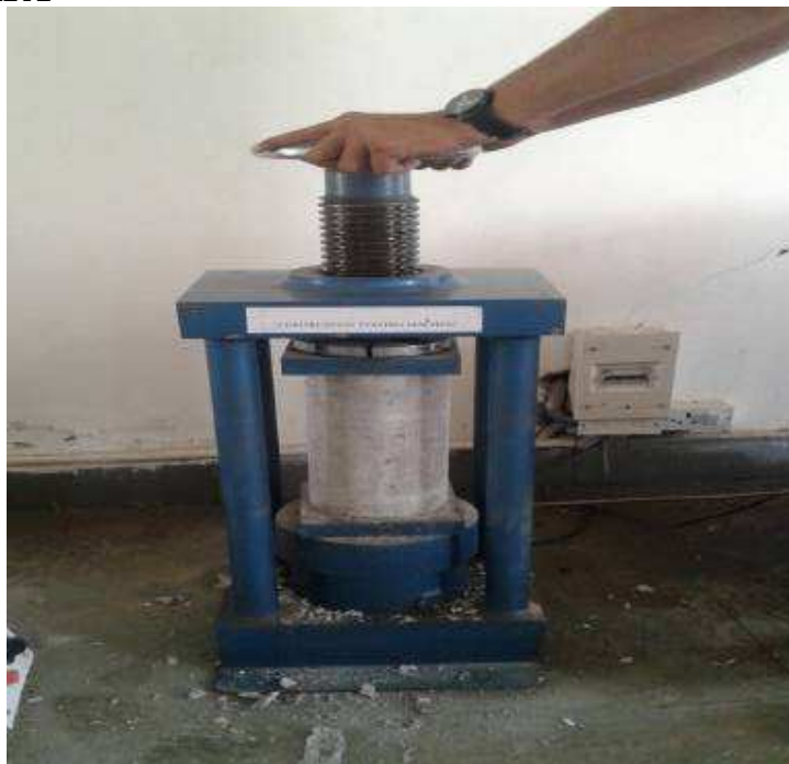
Fig 3.2 Test Set up for Split Tensile Strength
