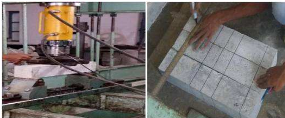
Fig 7.5: schematic representation of a) flexural strength test b) marking of specimen
