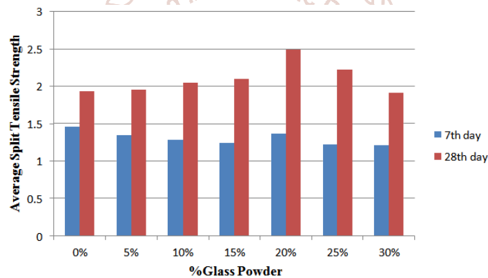
Fig 8.3 Comparison of Split tensile strength of M30 concrete on 7th and 28th day curing periods
