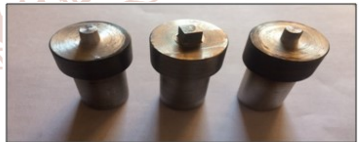
Figure 5.3 - FSW tool with tapered, square & cylindrical pin
