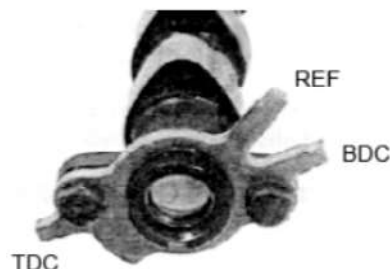
Fig.2.6 Camshaft Position sensor's cog detail
