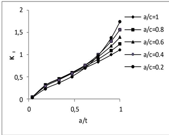
Fig. 7. Variation of SIF at the surface point using six term weight function.
