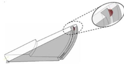
Fig. 4. Semi elliptical crack at blade mounting location
