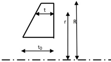
Fig. 1. Tapered rotating disc
