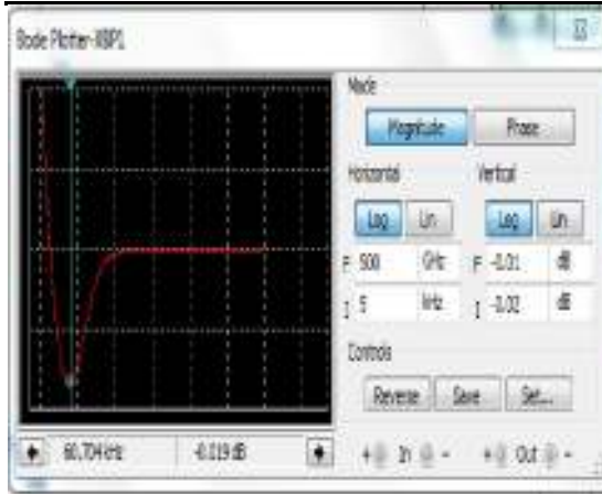
Fig.4(a): frequency response curve of BRF circuit
