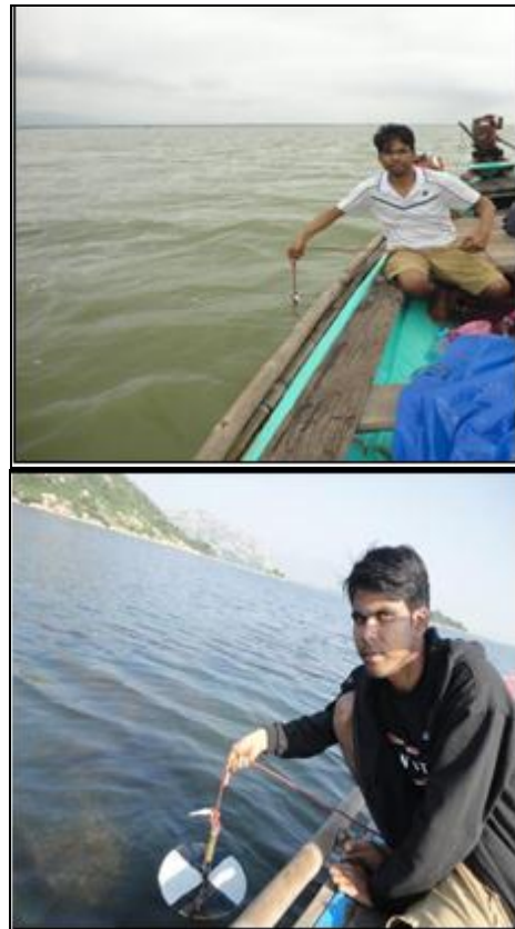
Figure 2. Use of Secchi disk in Chilika Lake
