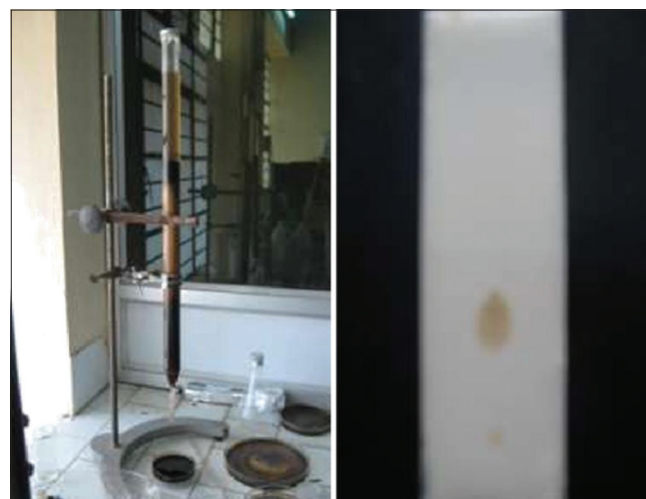
Figure 1: Separation of alkaloids by column chromatography
