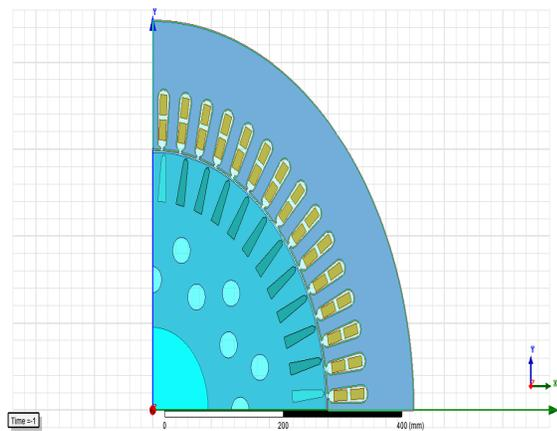
Fig.6 Maxwell 2-D geometry of designed motor
