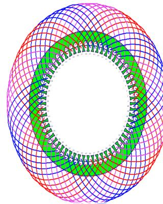
Fig.4 Winding arrangement view in RMxprrtool
