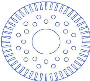
Fig.2 Rotor model of 48 slots developed in RMxprrtool
