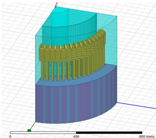
Fig.7 Maxwell 3-D geometry of designed motor
