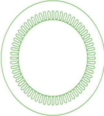
Fig.1 Stator model of 60 slots developed in RMxprrtool
