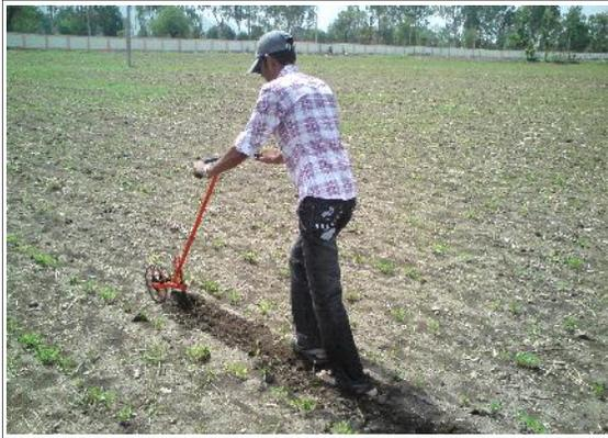
Fig. D : Field testing of the weeder
